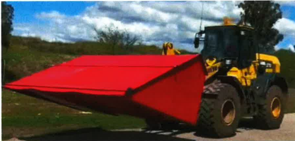
Figure 6: An LBin fitted with a quarantine membrane to receive and contain hazardous materials.
